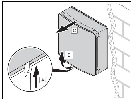
3. Remove the fan unit with wind guard and front panel.
